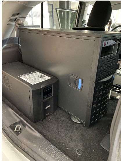
Figure 3.4: ATLASCAR2 processing unit and UPS
